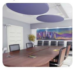
Plaka-dBound Raft is designed to absorb sound and enables to achieve the optimum level of acoustic comfort, prevents echo and reverberation and ensures enhanced speech intelligibility.
