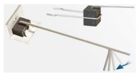
The acoustical wall tie is composed of 3 elements: a stainless steel holder, a rubber block (cork- elastomer – 30x30x25mm) and a one-sided folded wall tie (ø4mm).
