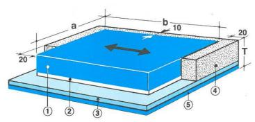
① EPDM bearing with TEFLON sliding sheet ②
