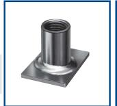
The PFEIFER flat steel anchor is one of the lifting anchors in the PFEIFER thread system. It is particularly suitable for thin plates. With the welded-on flat steel and an appropriate tensile reinforcement on top, safe load application into the structural element is assured.
