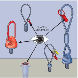
Check the system consistency by, for example, inspecting the data clip of the lifting anchor and the load capacity identification tag of the lifting loop.
