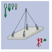
Warning: The use of non-matched system components can cause reduced safety levels and hazards to life and limb. Always use PFEIFER components that are matched to each other!
