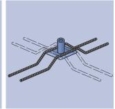
From size Rd 24 the reinforcements are installed crosswise – see illustration.
