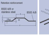
**Notice:** In the case of the waved anchor, short, and bolt anchor, no additional retention reinforcement should be installed.
