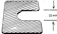
Plastic shims consist of a square plastic plate with dimensions 70 x 70 mm.
