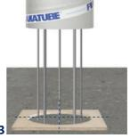
• For heights up to 4 meters, and if these installation instructions are carefully followed, it is not necessary to add an intermediate locking plate.
