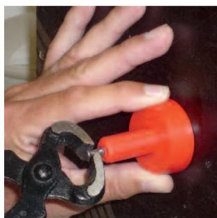
An easy removing off the nailing flange by the double headed nail
