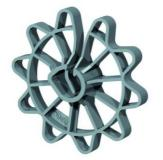
STAR is a spacer for a vertical reinforcement, made out of polyethylene.Due to its special design, STAR suits various bar diameters.Its open structure allows optimal flow of concrete.Its toothed structure allows the STAR to remain in place during the pouring and the trilling of the concrete.
