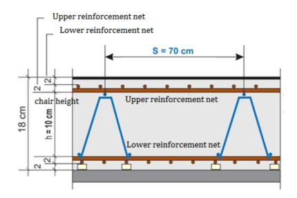
Thickness floor slab + 18 cm
