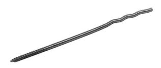
The masonry tie for timber frames is straight and has a threaded end, allowing anchoring in the interior wooden structure. The tie has a wood thread and screws directly into the frame. Anchoring in the masonry is ensured by the wave at its other end.
